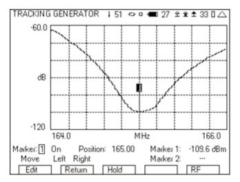
Figure 35 - Zooming in to the reject band of the duplexer
