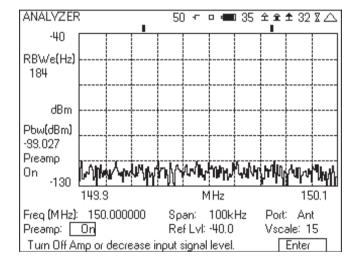
Figure 37 - Analyzer screen showing input overload condition
