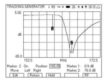
Figure 32 - Tracking Generator with markers
