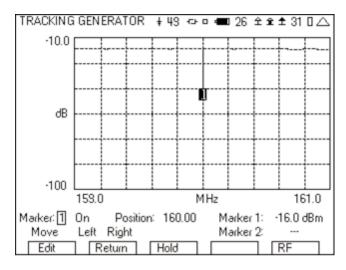
Figure 34 - Pass band loss
