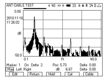
Figure 27 - Distance to Fault showing end of cable
