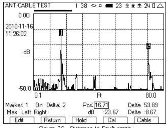
Figure 26 - Distance to Fault graph
