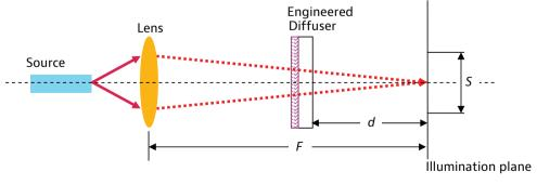
Figure 3. Sharp spatial cutoff illumination system with controlled image size. The lens focuses at the illumination plane and the diffuser is placed between the lens and the illumination plane.
