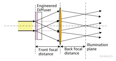
Figure 5. **Telecentric illumination system with Engineered Diffuser.** Finite collimated illumination beam is depicted. The figure illustrates three individual field angles. One axial and two other extreme collimated ray bundles are shown leaving the diffuser and forming sharp features at the back focus of the lens.
