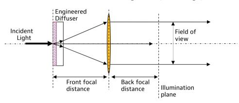
Field of view = focal length  $\times$  tan (diffuser angle).
