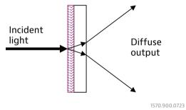
Figure 1. **Simple diffuser application.** Shown is a beam of light incident on the patterned side of the Engineered Diffuser. Light is refracted at the surface into the substrate. Upon exiting the substrate the light refracts at the planar surface achieving the designed angular spectrum.
