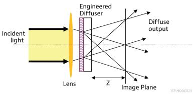
Figure 2. Sharp spatial cutoff illumination system. The diffuser is placed near the pupil of the lens system following the lens.
