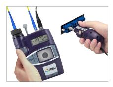
Inspect the Patch Cord with Integrated PCM and the Bulkhead with Probe
