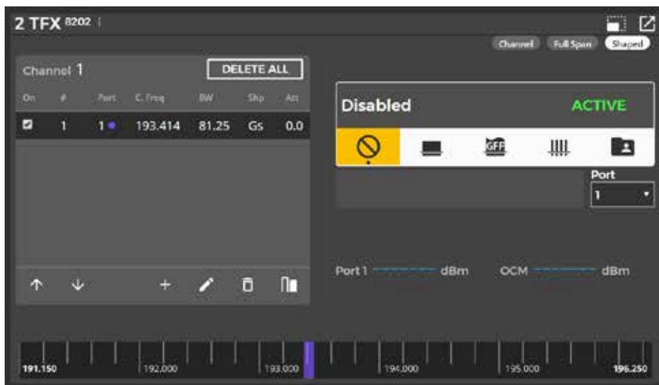
Figure 9 – Shape mode displayed on the MAP-300 GUI
