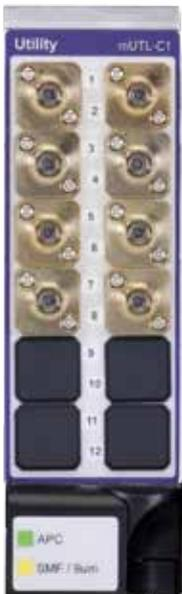
The mUTL-C1 cassettes simplifies the mechanical integration of passive optical components for test sets. They are highly configurable, contain passive optical devices such as splitters and taps. They support angle or flat polished connectors as well as single-mode and multi-mode fibers. Each module has user definable data fields that can be accessed by the MAP series chassis to assist in module identification and displayed or recalled remotely.
