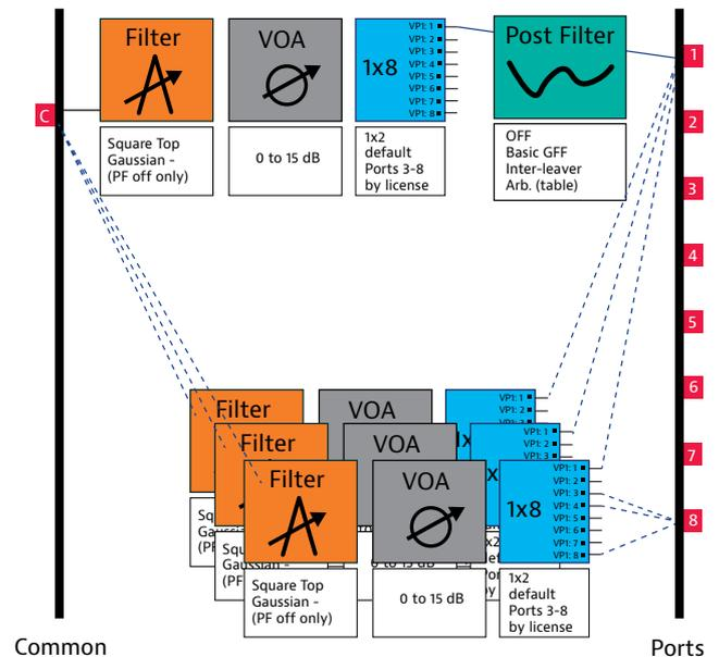
Figure 2 - The mTFX-C1 showing individual control blocks
