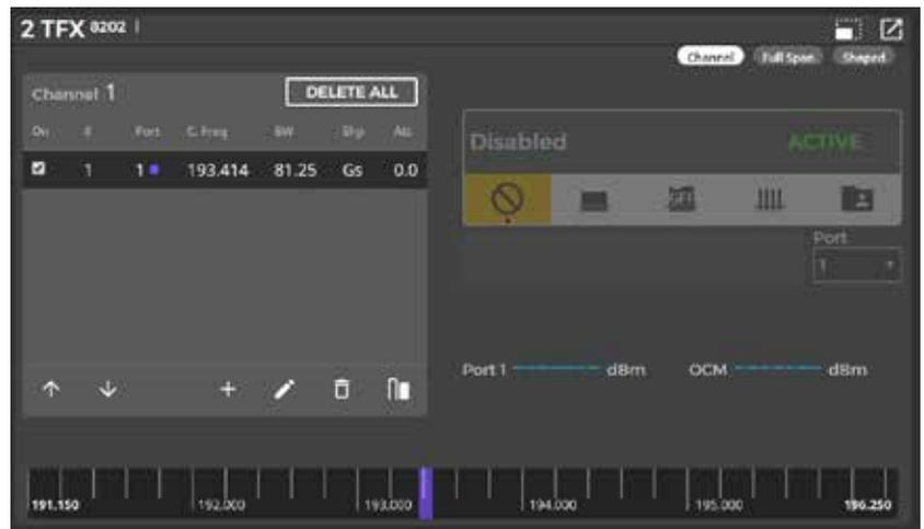
Figure 5 – Channel mode displayed on the MAP-300 GUI
