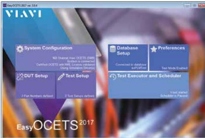
Simple, clear interface makes checking status or training new operators fast and efficient. Tool sets for adding setup instructions make creating tests simple and efficient. Central database allows data to be accessed anywhere and test scripts to be programmed remotely.
