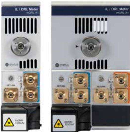
Multimode modules are based on the same basic technology and architecture as the single-mode module described above. A standard dual-wavelength version is available (850, 1300 nm) for multimode applications with an integrated power meter and optional 2x2 optical switches for automated bidirectional testing.
