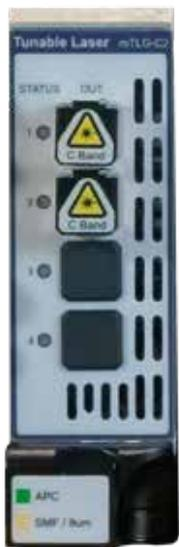
The mTLG-C2 is based on a Sampled Grating Distributed Bragg Reflector (SG-DBR) laser with an integral wavelength locker. Wavelength and output power settings can be controlled using the MAP series local interface or automation interfaces. The integrated wavelocker and automatic power control loop provide stable operation. The mTLG-C2 module is a new generation tunable laser module, which is ideal for DWDM testing where the capability to change wavelength on demand over the C and L
