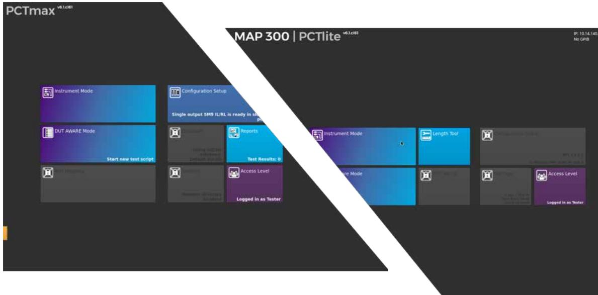
The PCT software has three main operation modes: instrument mode, script mode (DUT aware mode), and port mapping. For more information on port mapping consult the port mapping application note. A full complement of SCPI compliant remote commands is available as well.
