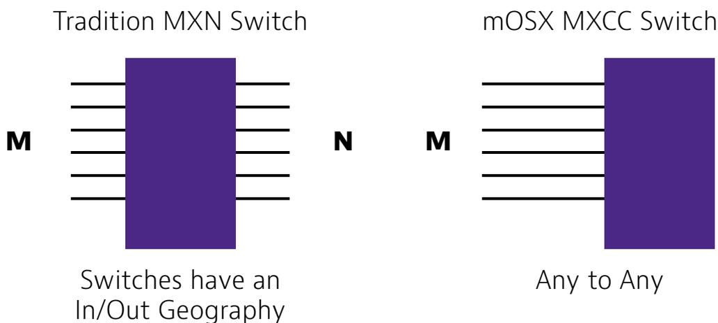
Figure 1. MxN switch topology have an inherent directionality. Ports on the M-side can connect to any N-side port, however M-side ports cannot connect to each other. In an any-to-any or “Common Connection” switch a port can connect to any other port
