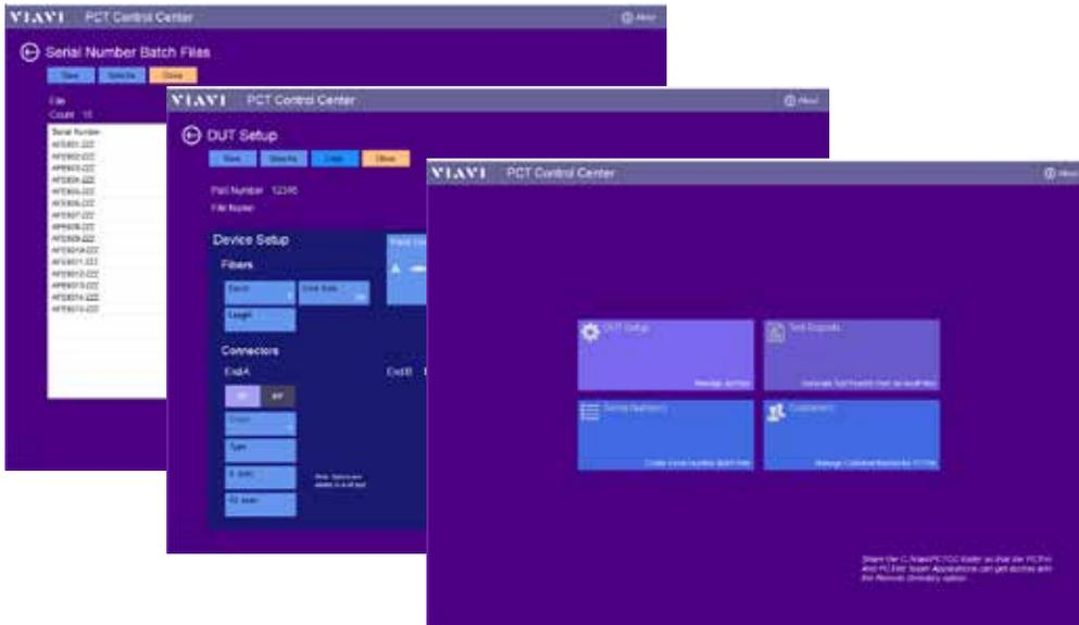
**PCT Control Center is a simple PC application designed to simplify management of the PCTMax, PCTLite and PCT-rm based IL and RL systems.**
