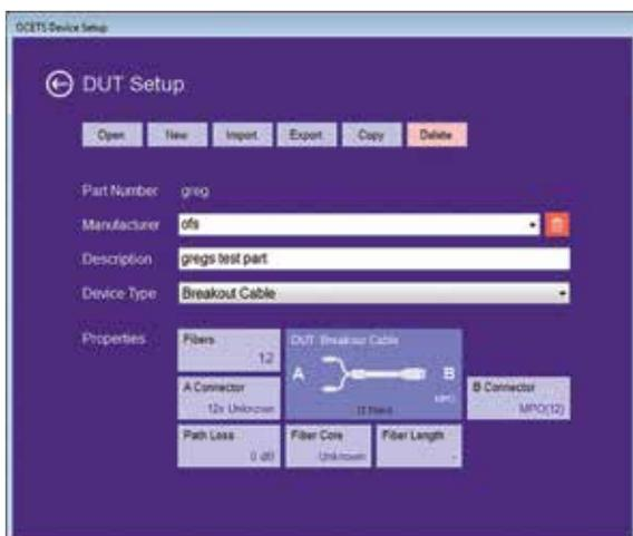
Device under test (DUT) libraries are created using a simple editor. Auto-channel-connection algorithms simplify creating test scripts.
