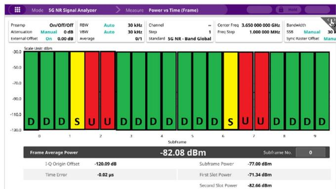
Figure 9: Over-the-Air Frequency and Time Error and Frame Synchronization measurement with the CellAdvisor 5G
