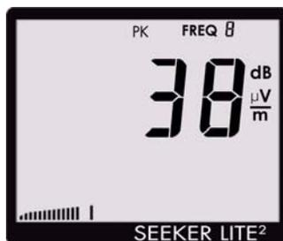
In the Preset Frequency display, the **FREQ** icon at the top of the display will blink and be followed by the preset frequency number.
