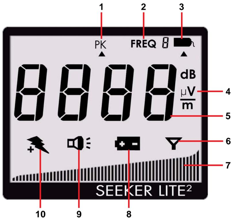
1. **PK** - This icon is shown when the Peak Hold feature is active. When the icon is not shown, the Peak Hold feature is turned off.
