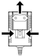
Fig. 3: AC line plug adapter
