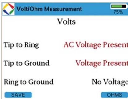
Indicates AC and DC voltages via the Volt/Ohm mode
