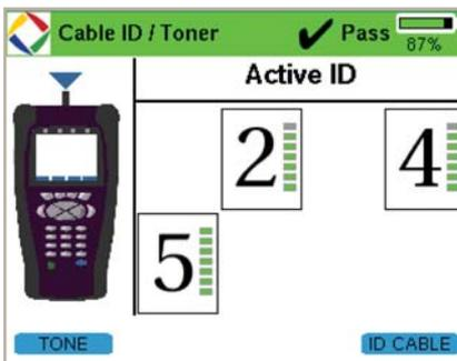
Cable ID mode with Active IDs lets technicians identify connections for each segment of coaxial cable
