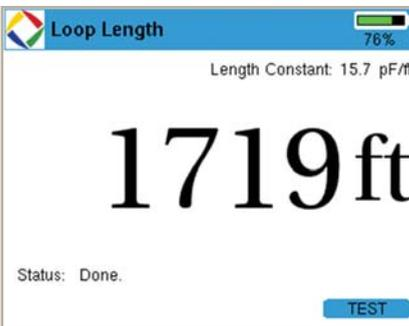
Loop Length test measures the length of unterminated twisted pair cables
