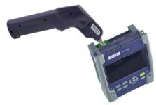
Figure 3: OTDR Port Inspection
