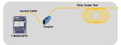
Figure 4: Connecting to coupler
