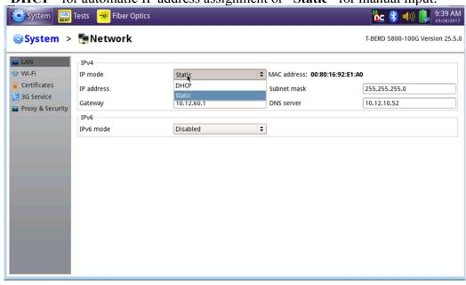
After configuring LAN settings, press the System icon, system, to redisplay the System Menu.
