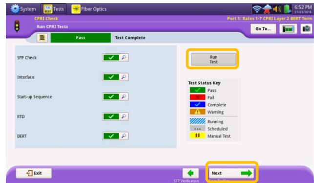
Figure 9: Run CPRI Tests screen
