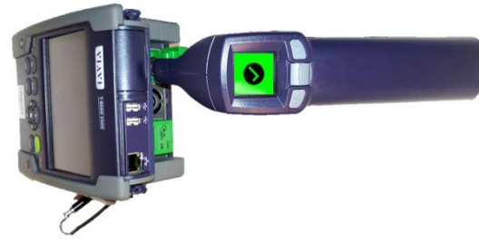
Figure 3: OTDR Port Inspection
