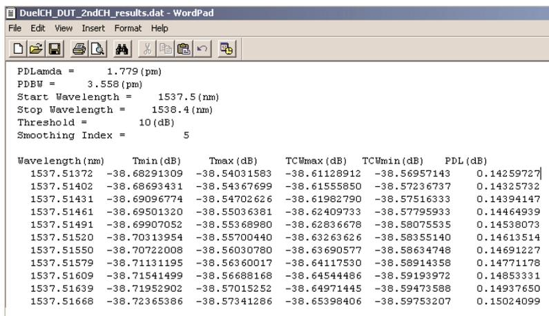
Figure 12. Output file of the analyzed TE/TM Loss
