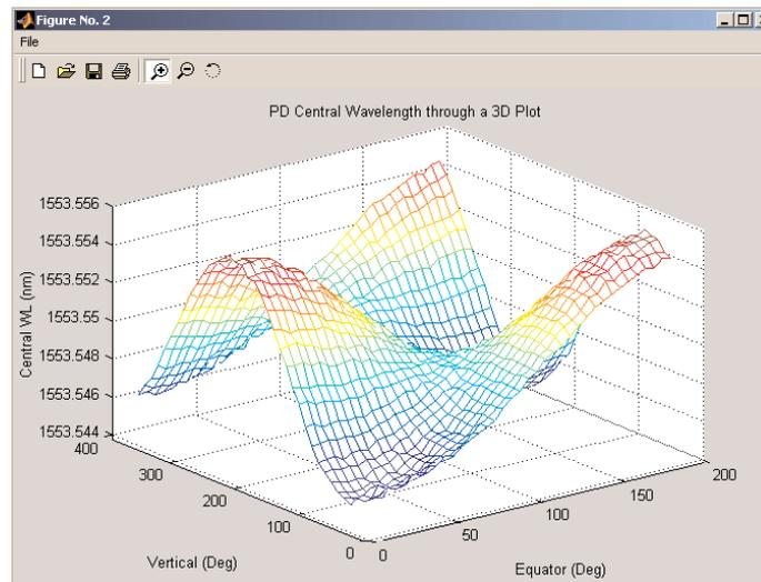
Figure 8. The polarization dependent CW across the Poincare sphere
