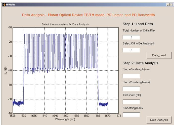
Figure 10. GUI for TE/TM loss application
