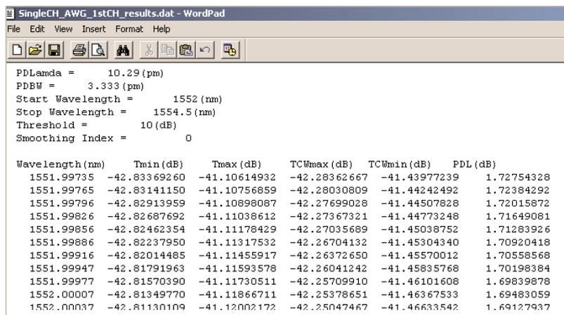
Figure 5. Output file of the analyzed TE/TM Loss
