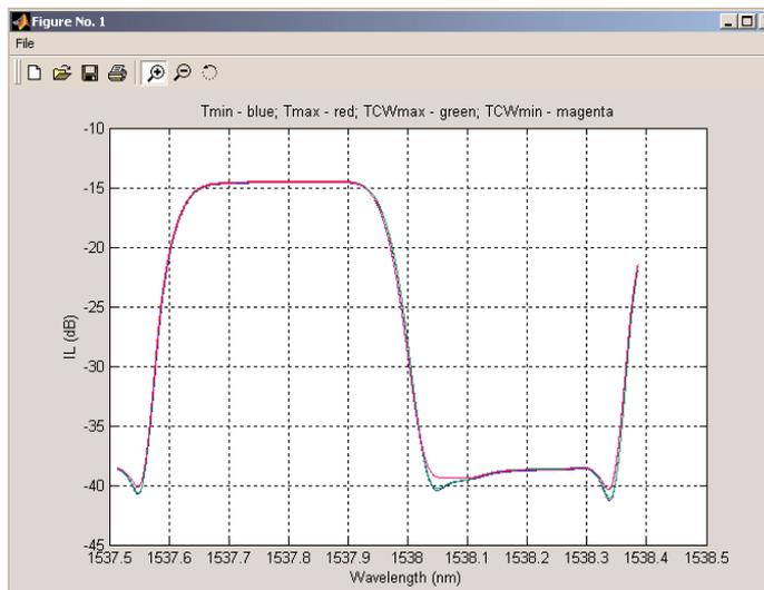
Figure 13. TCWmax and TCWmin correspond to TE/TM Loss
