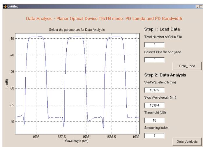
Figure 11. Zoom the analyzed area and input the data analysis parameters
