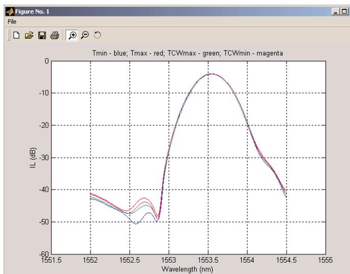
Figure 6. TCWmax and TCWmin correspond to TE/TM Loss
