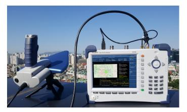
To meet trial deadlines, the VIAVI NEM partner was not able to remove the source of interference. Instead, they used CellAdvisor measurements to relocate the radio head. Consequent measurements indicated a reduced level of interference near the new location. The radio was brought back in service. This let our NEM partner complete their customer proof-of-concept in a timely manner.
