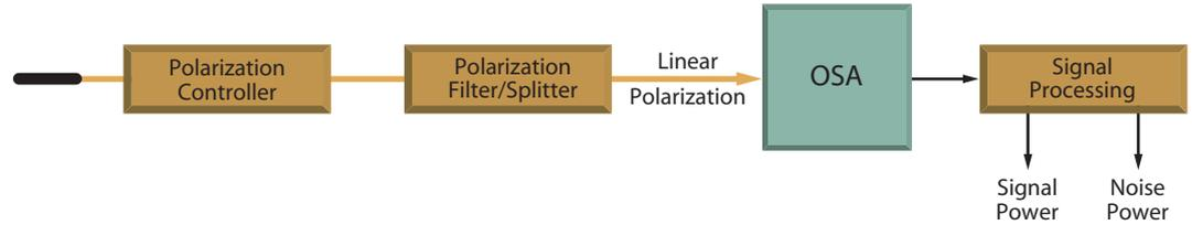
Figure 3 A block diagram of the OPS method
