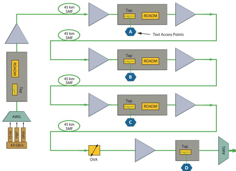
Figure 4 Block diagram of test setup at Tellabs/Chicago
