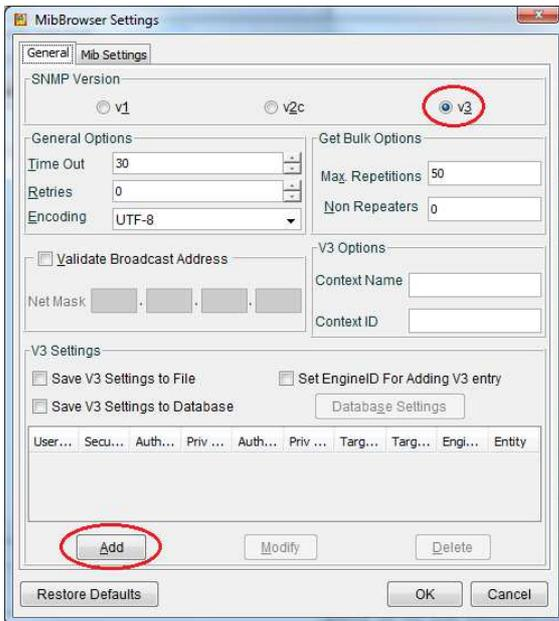
**WARNING:** because MIB Browser Free Tool checks the user configuration with the SNMP agent, ONMSi SNMP should be up and running. You won't be allowed to add an SNMP user in MIB Free Tool if the entered configuration does not match the `jdmk.security` and `jdmk.uacl` configuration files!
