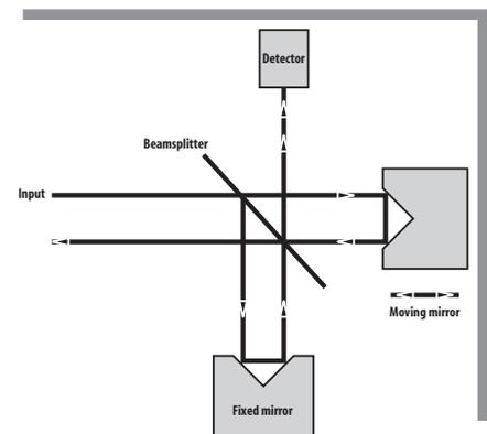
figure 1 Interferometric method
