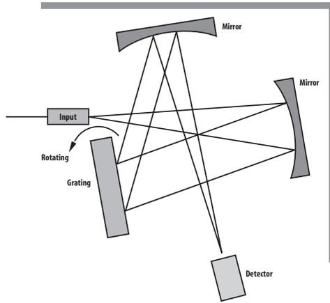
figure 2 Diffraction grating
