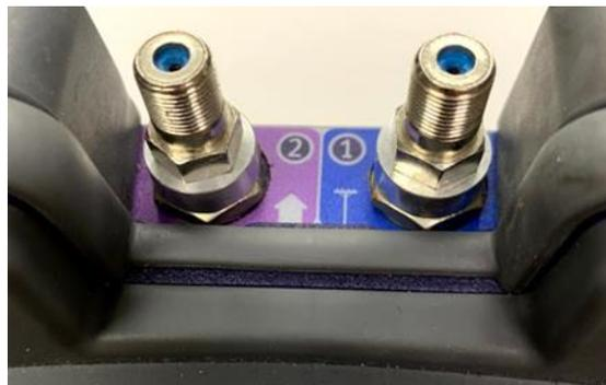
**WARNING:** Do NOT overtighten the F-81 adapter into the ONX's RF port, this can lead to permanently broken RF ports. Also, it is not recommended to use power tools when removing or replacing the F-81 adapters.
