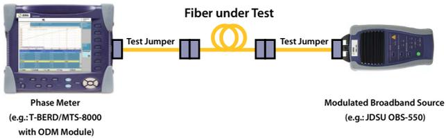
Figure 84: CD test setup with the JDSU solution
