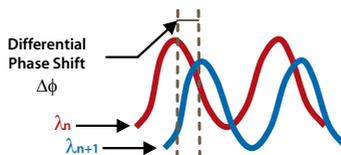
Figure 31: Schematic of Differential Phase Shift measurement
