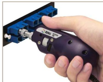
Figure 72: Bulkhead inspection
