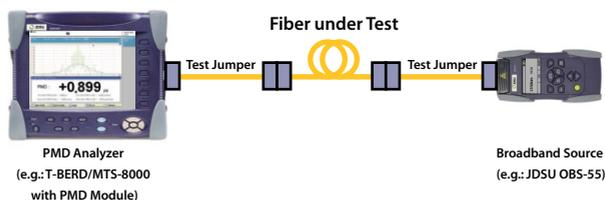
Figure 86: PMD test setup with the JDSU solution
