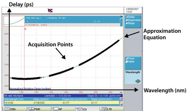
The CD is computed by calculating the slope of the group delay curve as a function of wavelength.
