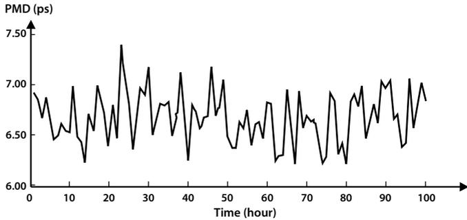
Figure 50: Long-term fluctuations of the average DGD
