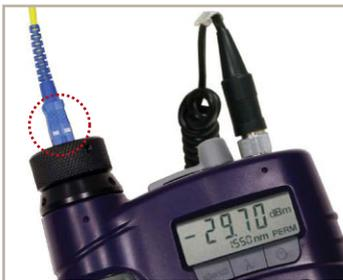
Figure 71: Patch cord inspection
