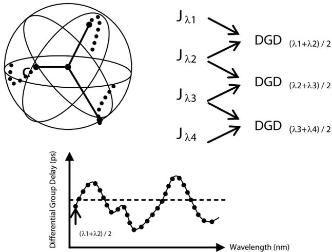
The accuracy at which the DGD can be determined increases with the frequency range within which the Jones matrix is analyzed. The frequency steps for the tunable laser have to be chosen carefully to match the expected DGD in the fiber.
