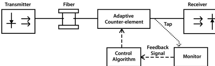
Figure 49: Schematic diagram of an optical PMD compensator
