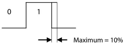
For example, 10 Gbps SONET/SDH transmission exhibits a bit length 100 ps which derives to a 10 ps maximum delay.
