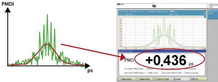
Figure 87: PMD measurement display with the JDSU Fixed Analyzer method in the T-BERD/MTS platform
