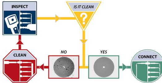
Figure 70: Connector inspection and cleaning steps
