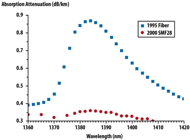
Figure 62: OH- absorption vs. fiber manufacturing time
