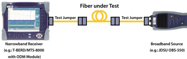
Figure 88: PMD test setup with the JDSU solution
