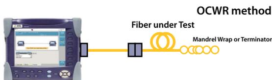
Figure 79:T-BERD/MTS-8000 with OFI module
