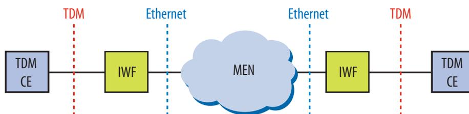
Figure 1. Transport of TDM Services over Packet Networks
