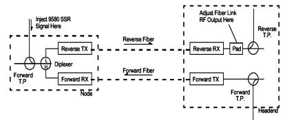
Figure 5. Return Fiber Link RF Output.
