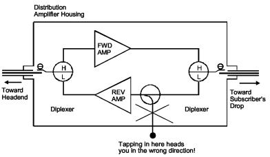
Figure 7. Incorrect Test Point Selection.
