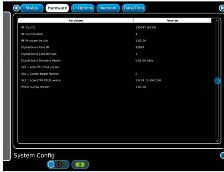
Fig. 5-8 System Config - Hardware
