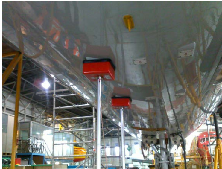
Fig. 4-14 ALT-9000 Antenna Coupler Installed
