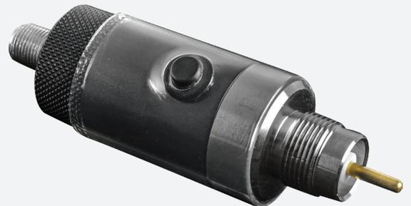
Simply screw the probe into a KS port on the distribution tap, connect the field meter to the test port, then press the button on the side of the probe. If the headend ingress displayed decreases by 4 to 6 dB when the button is pressed, the source of the ingress is farther from the node than the test point. Ingress that does not decrease is entering the system nearer to the node than the test point. The I-Stop probe has little or no visible effect on forward path signals.
