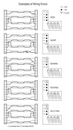
**Main Unit Results** – The main unit indicates the beginning of a test by flashing the pair lights in sequence top to bottom. The cable is then tested and the results displayed as follows:
