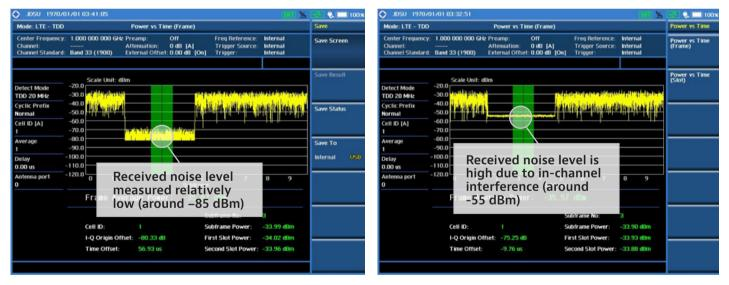
Figure 21a. Power vs. Time (Frame) plot of a LTE-TDD signal
