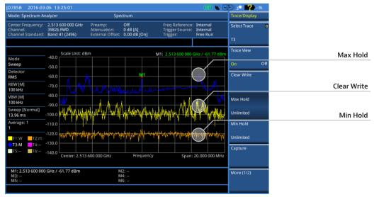
Figure 6. LTE-TDD signal in Spectrum Analyzer mode showing different trace modes
