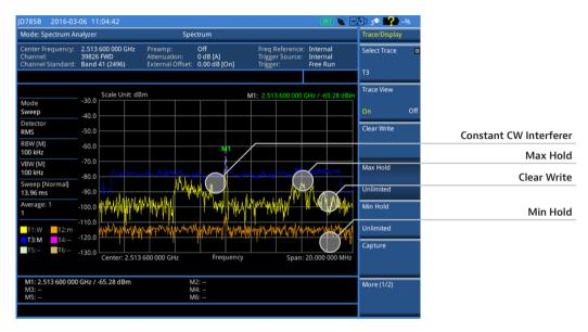
Figure 5. LTE-TDD signal in Spectrum Analyzer mode showing different trace modes
