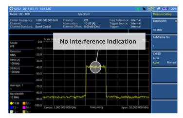
Figure 22a. Spectrum of Subframe 1 showing no presence of interference during the timeslot
