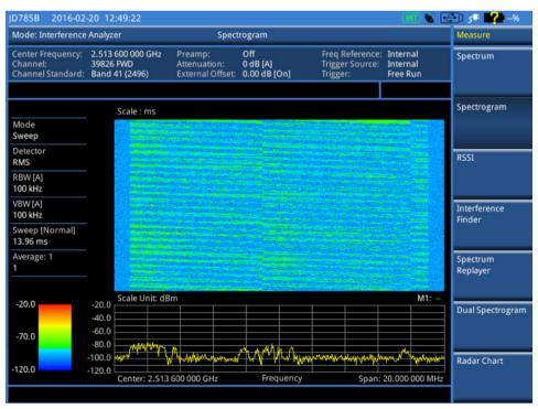
Figure 13. Spectrogram view of a 20 MHz LTE-TDD signal with no interferers (non-gated)
