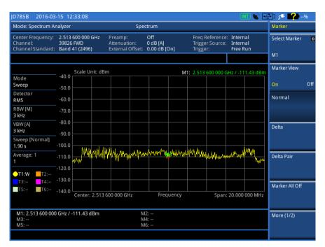
Figure 3. Stable LTE-TDD spectrum
