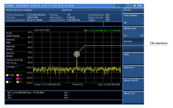
Figure 12. LTE-TDD signal in gated sweep mode, showing CW interference in the uplink
