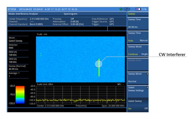
Figure 18. Spectrogram view in gated sweep mode showing CW interference in the uplink
