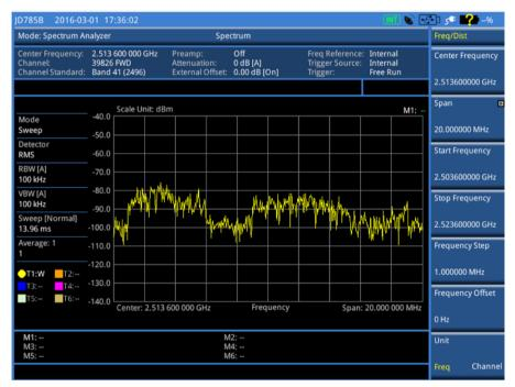
Figure 2. Spectrum of a 20 MHz LTE-TDD signal
