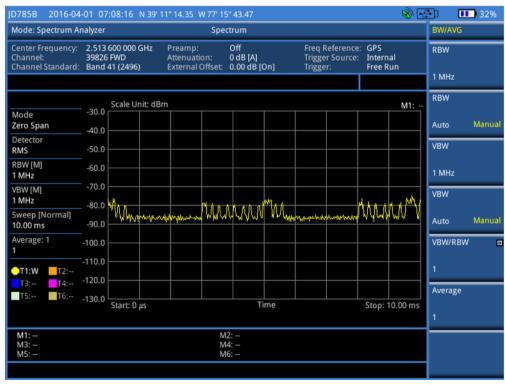
Figure 7. LTE-TDD signal in spectrum analyzer – zero span mode
