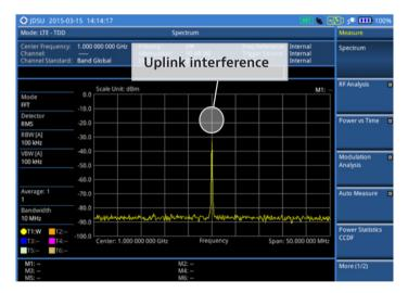
Figure 22b. Spectrum of Subframe 3 showing interference during the time slot
