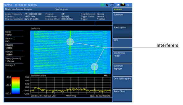
Figure 14. Spectrogram view showing intermittent interferences within the channel
