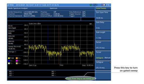
Figure 10. GPS triggered TD-LTE signal in spectrum analyzer zero span mode showing gated sweep settings
