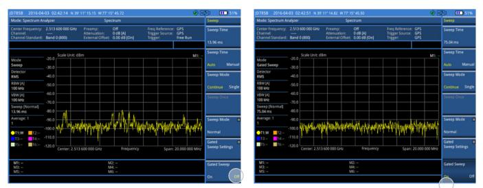
Figure 11a. LTE-TDD spectrum with gated sweep set to off
