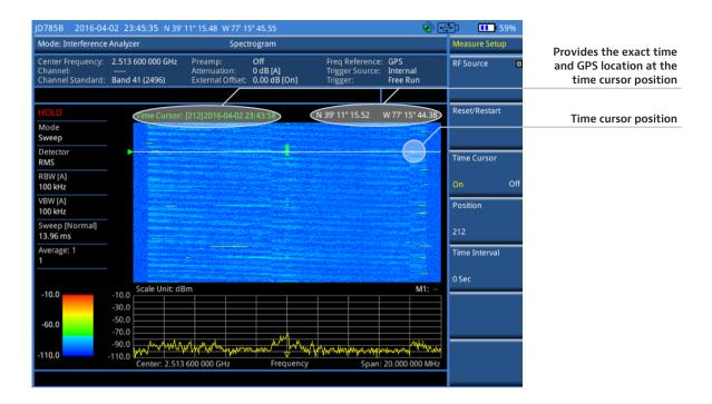
Figure 16. Spectrogram view showing time and location of interferer using the time cursor
