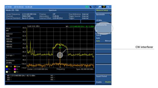
Figure 20. Spectrum view of subframe 0 in the LTE-TDD signal analysis mode
