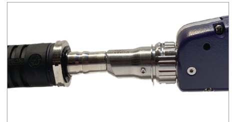
Sidewinder with FCPT-QODC2-S inspecting one of the sockets in a Q-ODC-2 socket connector
