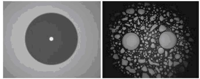
Figure 4. Microscopic views of clean connector end faces Fiber Connector Inspect/Clean/Connect Process
