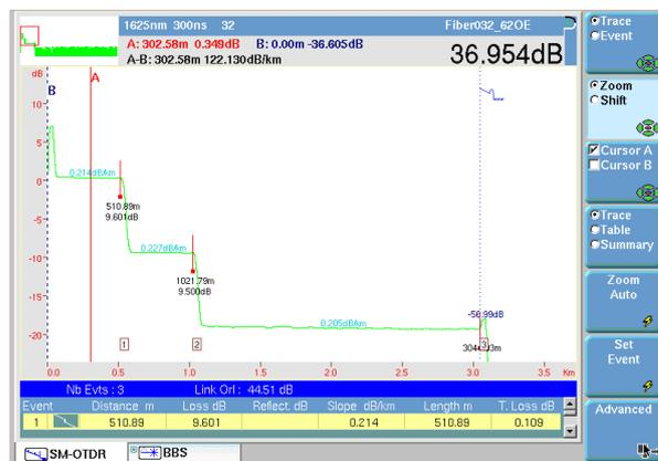
Figure 14. Cascaded splitter network test from ONT, without launch cable
