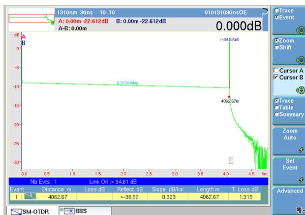
Figure 13. Distribution test only from ONT to first splitter, without launch cable
