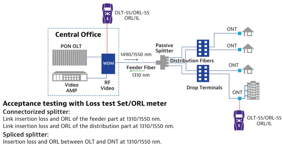
Figure 17. Qualifying the FTTH network with a loss test set/ORL meter
