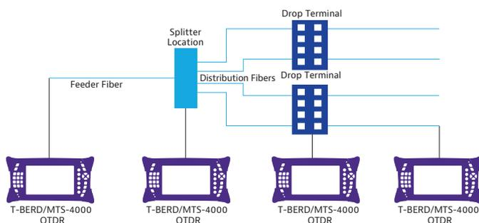
Figure 1. Possible access points for FTTH network qualification
