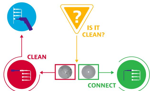
Figure 5. Optical connector Inspect/Clean/Connect Process
