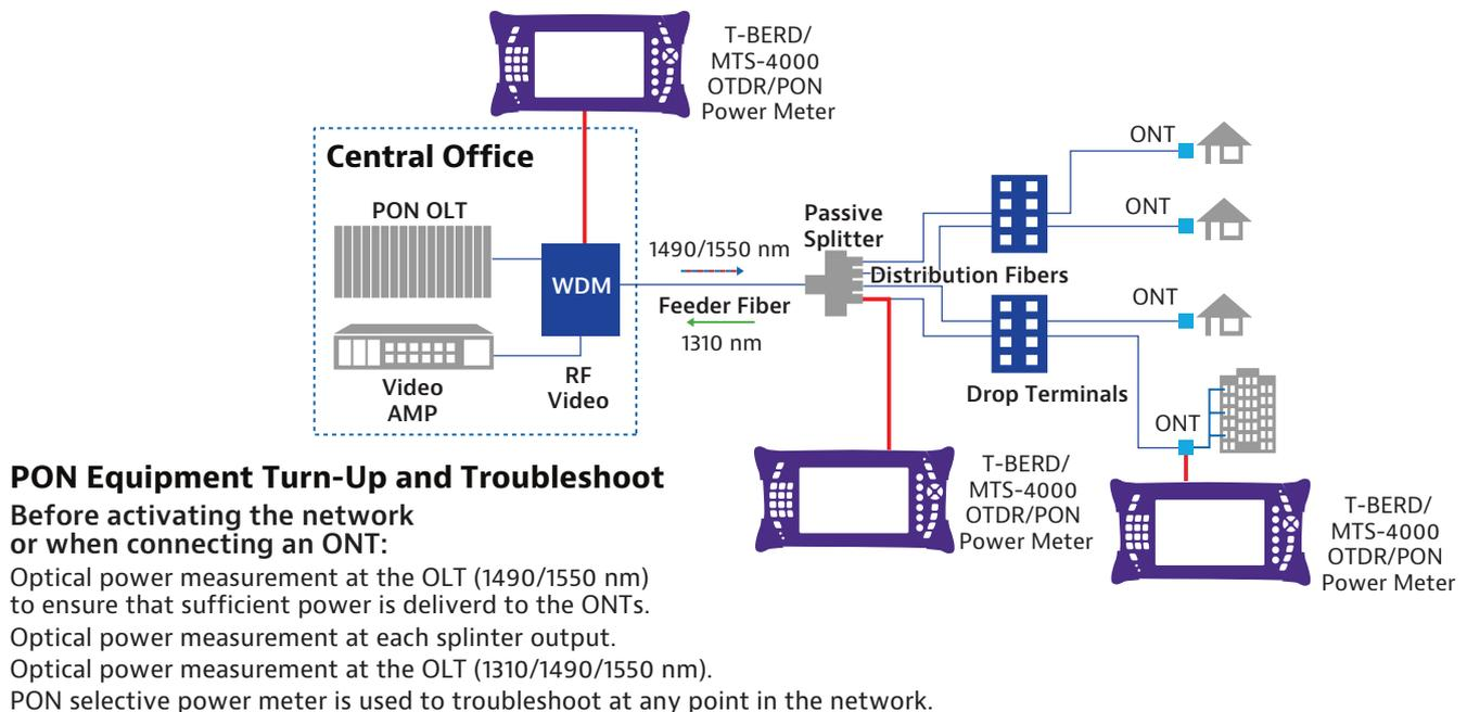
Figure 18. FTTH Network turn-up optical tools
