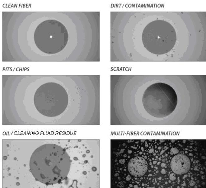
Figure 3. Fiber connections and various connector end face views as seen through an inspection scope. Ideally the fiber end face should be free from defects or scratches as Figure 4 shows.
