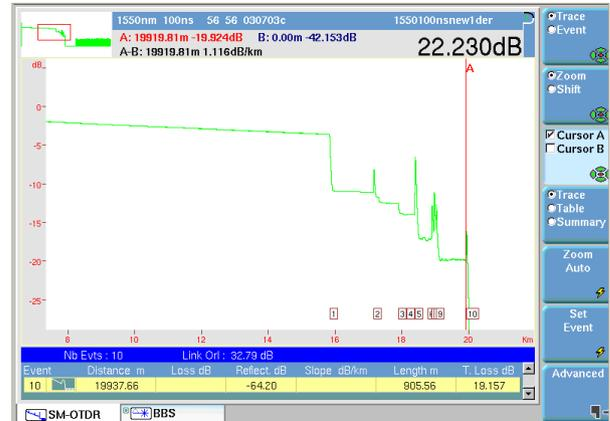
Figure 16. Cascaded splitter network test from OLT, without launch cable
