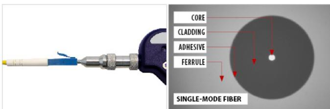
Figure 6. Patchcord microscope inspection
