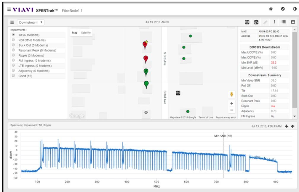
In addition, these new solutions handle all common use cases including ingress remediation, sweep and leakage tagging while interacting in real-time with field testing units. This allows technicians see the results of their efforts in real-time to get the problem fixed as quickly as possible.
