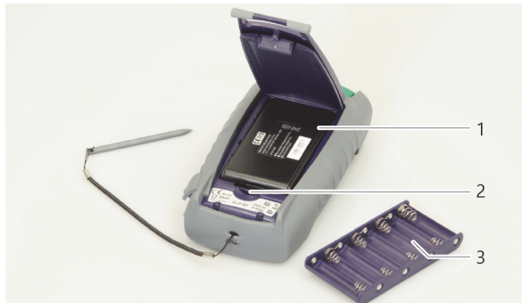
Fig. 4 Replacing the batteries
