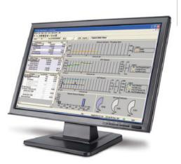
Figure 1. The Triple Play Analyzer dashboard shows traffic distributions and top-level performance for voice, video, and data services
