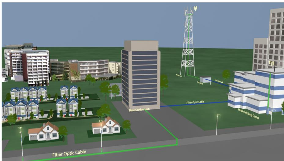
The fiber link between the BBU and RRU, AKA the “front-haul,” carries RF information using either CPRI or OBSAI technology. Basically, RF information from the radio is converted into the digital domain and mapped accordingly so that it can be deciphered at the BBU and vice versa.
