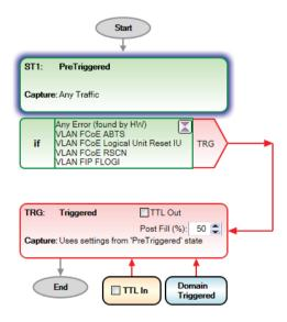
Figure 4. TraceControl trigger/filter configuration
