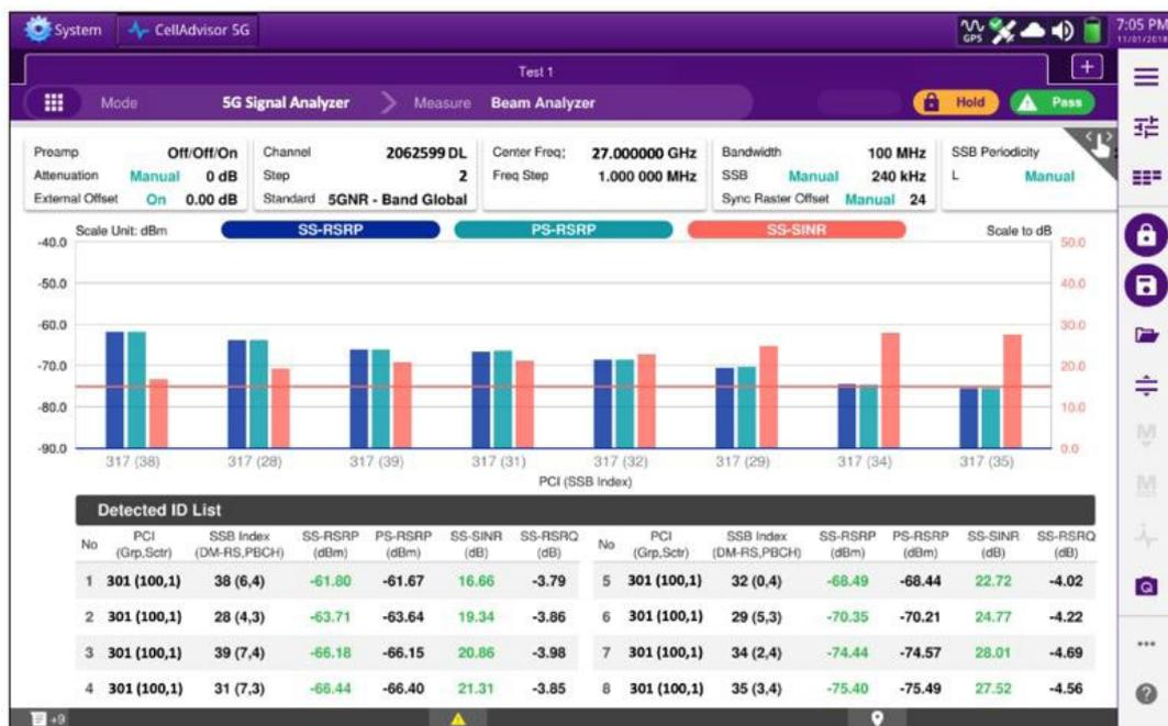
Figure 10: CellAdvisor 5G Beam Analyzer (8 strongest beams)
