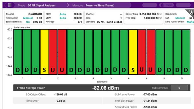
Figure 9: Over-the-Air Frequency and Time Error and Frame Synchronization measurement with the CellAdvisor 5G
