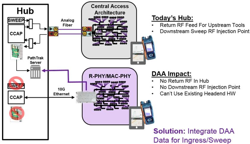
Figure 8 Integrate DAA Data Into OSS
