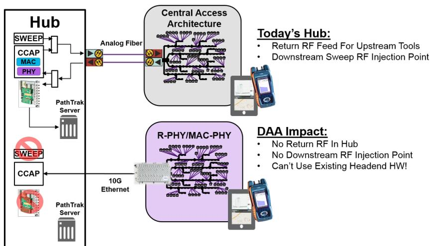
Figure 6 RF Test Points Removed from Hub with DAA
