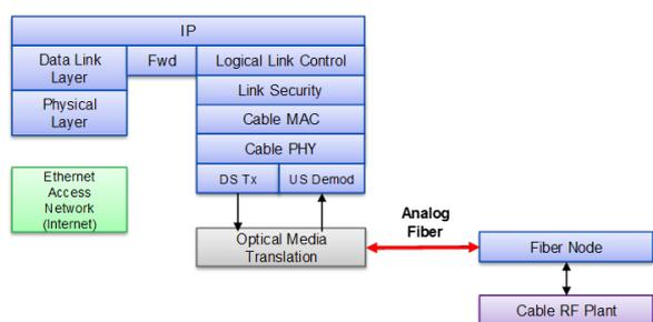
Figure 1 Current - Centralized Access Architecture
