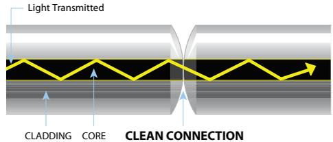
Today's connector design and production techniques have eliminated most of the challenges to achieving **core alignment** and **physical contact**.
