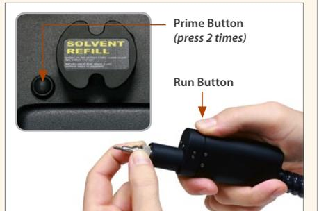
2. Insert the handset into the bulkhead and push to disengage safety mechanism (*the POWER/READY light will turn green*), and press the **run button** to initiate cleaning.
