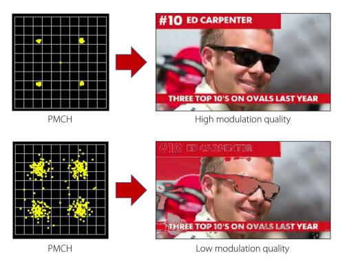
Figure 8. Broadcast (MBMS) modulation quality
