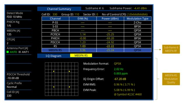
Figure 10. CellAdvisor MBMB SFN reference signal (MBSFN RS)
