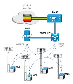
Figure 2. MBMS network architecture
