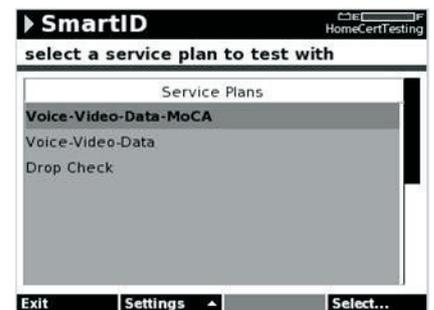
A supervisor can edit, add to, or delete service plans from any DSAM using TPP and can push them to any or all DSAMs.
