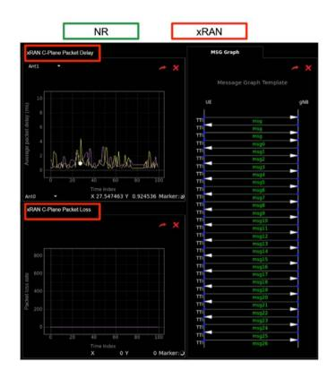
Figure 4: TM500 Lab to Field Dashboard showing packet loss and delay
