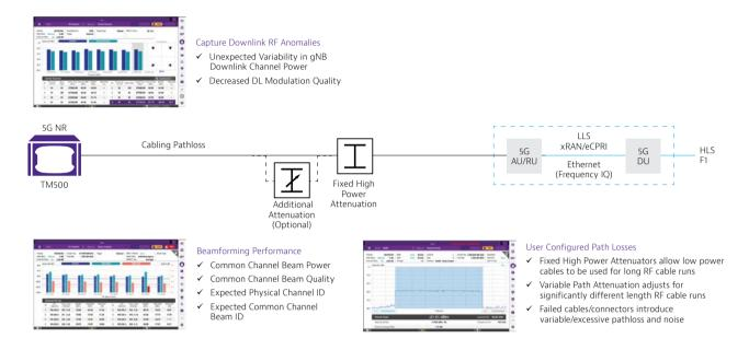
Figure 2: TM500 and CellAdvisor5G Lab to Field Solution
