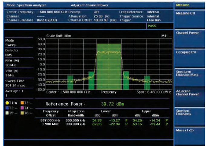
RF analysis — Adjacent Channel Power
