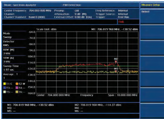
RF test — PIM Detection
