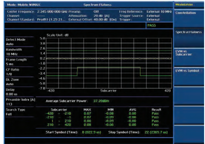
Modulation analysis — Spectral Flatness
