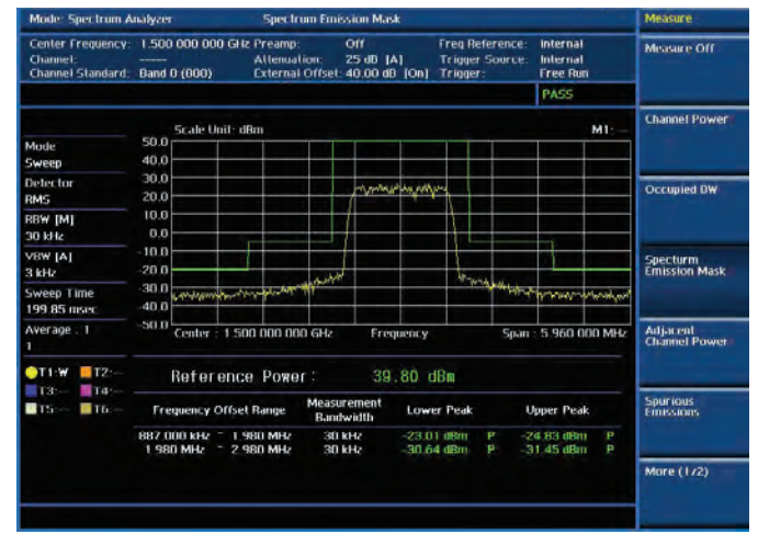
RF test — Spectrum Emission Mask
