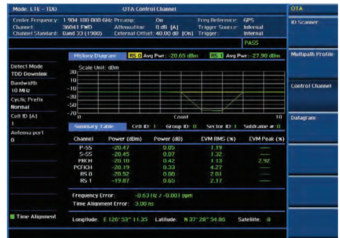
OTA analysis — Control Channels
