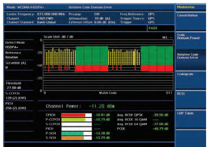
Modulation analysis — Relative Code Domain Error
