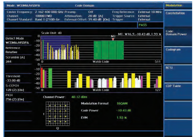
Modulation analysis — Code Domain Power
