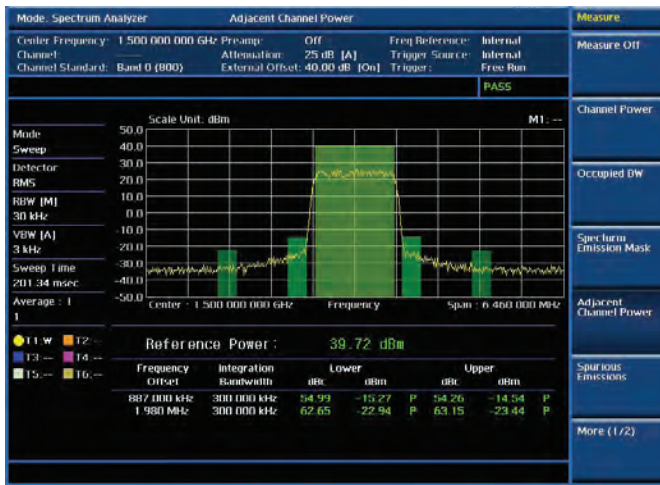
RF test — Adjacent Channel Power
