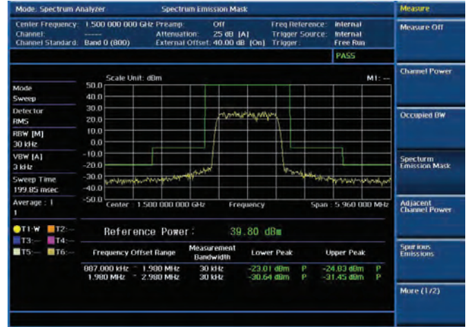
RF analysis — Spectrum Emission Mask
