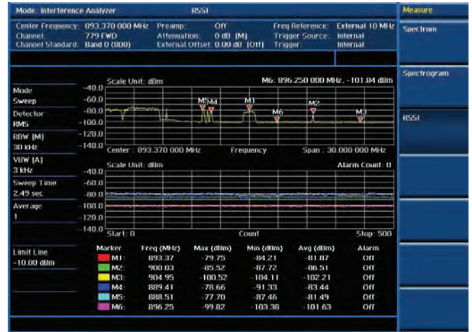
Interference analysis test — RSSI
