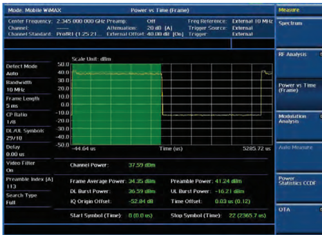
Modulation analysis — Power vs. Time (Frame)
