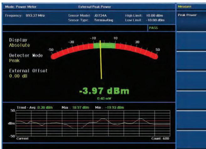
Power meter test (RF or optical)
