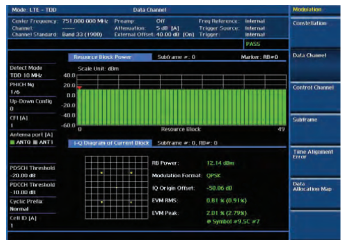
Modulation analysis — Data Channels
