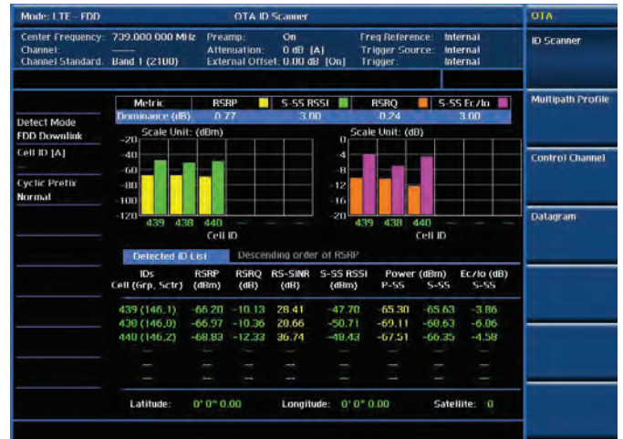
OTA analysis — ID (Channel Scanner)
