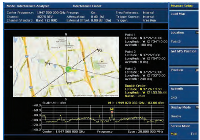
Interference analysis test — Interference Finder
