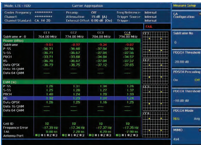
Modulation analysis — Carrier Aggregation
