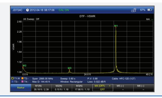
Figure 3: Distance to Fault measurement (VSWR)
