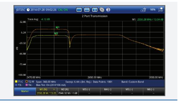
Figure 4: Insertion Loss Test view
