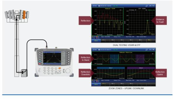
Figure 5: Cable and Antenna Test
