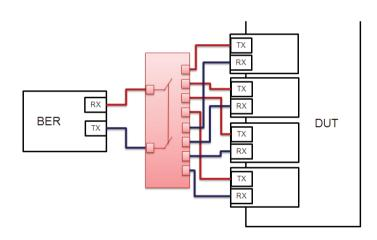
Figure 8. Converting a two 1Cx4 system to a single 2Dx4 system
