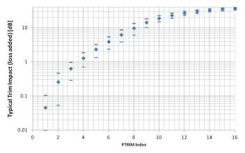
Figure 2. Typical PTRIM impact for 1CxN with 24 ports or fewer
