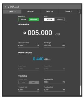
Figure 2 - mVOA MAP-300 detailed view GUI
