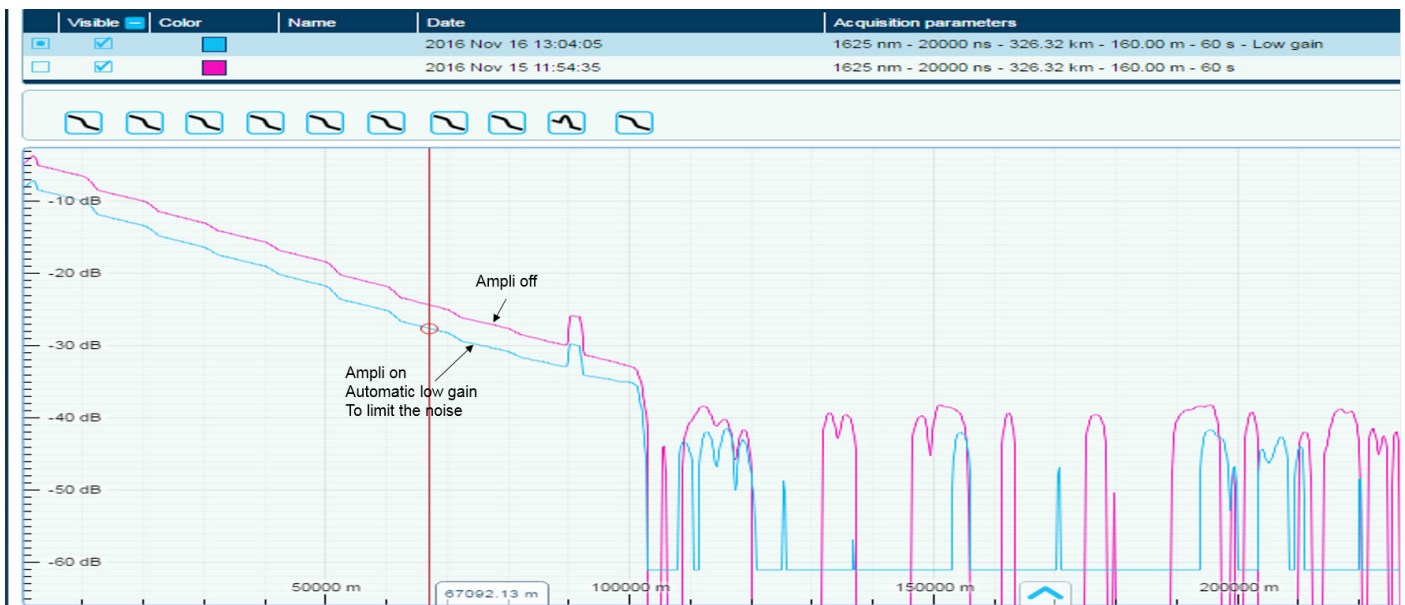
Figure 7: OTDR trace of contra-propagation with Raman amplifier
