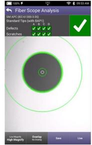
Figure 13: Passing Test
