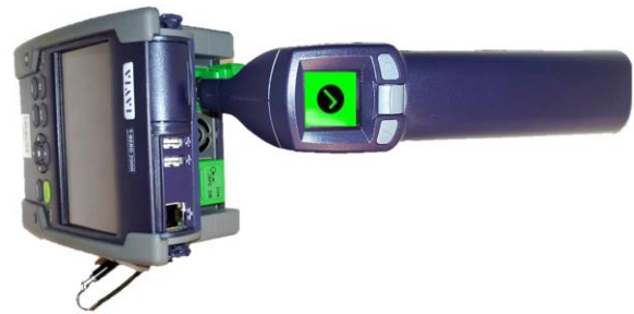
Figure 3: OTDR Port Inspection
