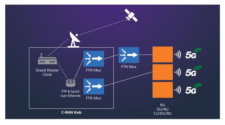
Figure 7: Timing distributed over 5G-NR network
