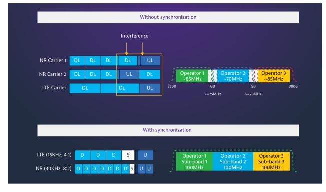
Figure 8: Frame synchronization
