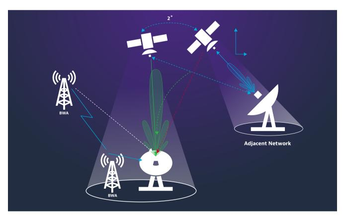
Figure 3: Interaction between satellite earth stations and broadband wireless nodes
