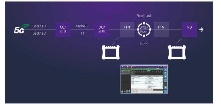
Figure 6: Example of 5G fronthaul RU connectivity and delay test
