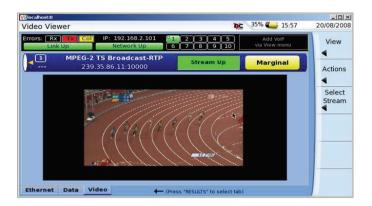
Figure 4. Example of IPTV Video Stream test
