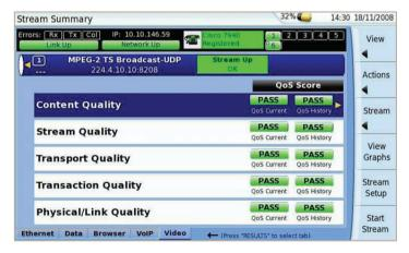
Figure 2. Example of Video test results using the T-BERD/MTS-4000 GUI with the Viavi Quality Layer Model
