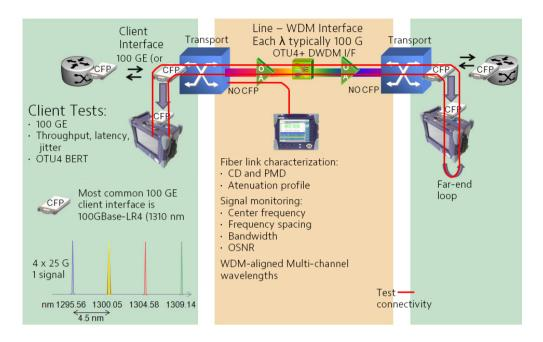
Figure 2. Line and client interfaces
