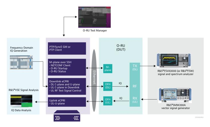
The VIAVI O-RU Tester NETCONF client supports stateful M-plane. The O-DU cycles through typical M-plane procedures and establishes a link with the O-RU. The O-DU emulator C/U-plane engine generates real-time eCPRI packets from downlink signal generated by Vector Signal Generator (VSG). eCPRI packets are transported to O-RU via Open Fronthaul interface. R&S®VSE Vector Signal Explorer software and Vector Signal Analyzer (VSA) support analysis of downlink signal from the O-RU Tx port.
