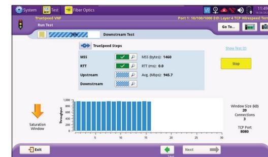
User sees real-time throughput measurements while test is running
