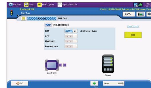
Using the VIAVI T-BERD/MTS-5800 with the RFC 6349-compliant TrueSpeed option, TCP tests can be run in less than 5 minutes by novice technicians using a simple, push-button interface.
